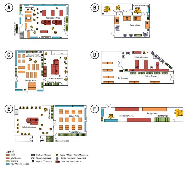
Figure 2. Floor Plans of the (A) Architecture Model Studio, (B) Digital Fabrication Studio, (C) First-Year Teaching Shop, (D) Grad Space, (E) Industrial Design Studio, and (F) Metal Foundry. Note that the floor plans are not to scale.
