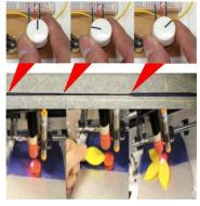
**Figure 10.** The connected a number of sensors enable the printer to control printing parameters, *i.e.* thickness of deposited lines real-time (Top). It can also guide human to enable inserting foreign items onto the object (bottom)
