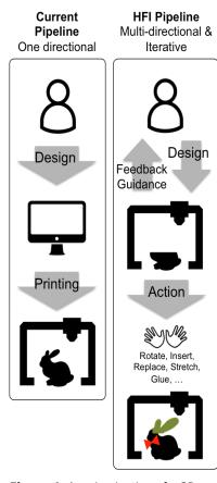
**Figure 4.** A re-imgination of a 3D printing workflow from the vantage of HFM Interaction. This proposed multidirectional process allows the user to modify their design during production, allowing for spontaneous decisions and ideas to be incorporated without needing to begin production from the beginning.
