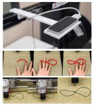
**Figure 9.** An early prototype of the Sensing Machine that captures users' gesture path and replicate 'drawing' with plastic. A leap motion tracks the human gesture, being connected to an Arduino to communicate with a 3D printer.
